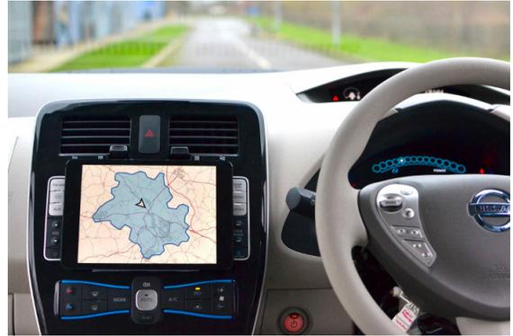
Fig. 1. Range map prediction installed in a real electric car showing destinations with estimated attainability probability at least 90%.
