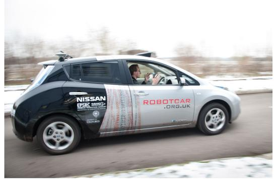
Fig. 6. The RobotCar (Modified Nissan Leaf) platform used for data gathering.
