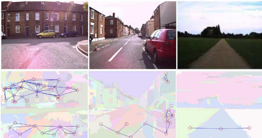
**Fig. 5** Typical graphs extracted from urban scenes as recorded by our mobile robot. **Top:** the original scenes. **Bottom:** the corresponding segmented images with the extracted graph overlaid. Circles indicate nodes, lines indicate edges. For images patches which are not marked as nodes no reliable geometry estimates could be extracted from the laser data.
