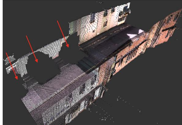
(a) Before: The *sparse* laser point cloud input after removing ephemeral objects (automobiles). The resulting gaps are highlighted by red arrows.
