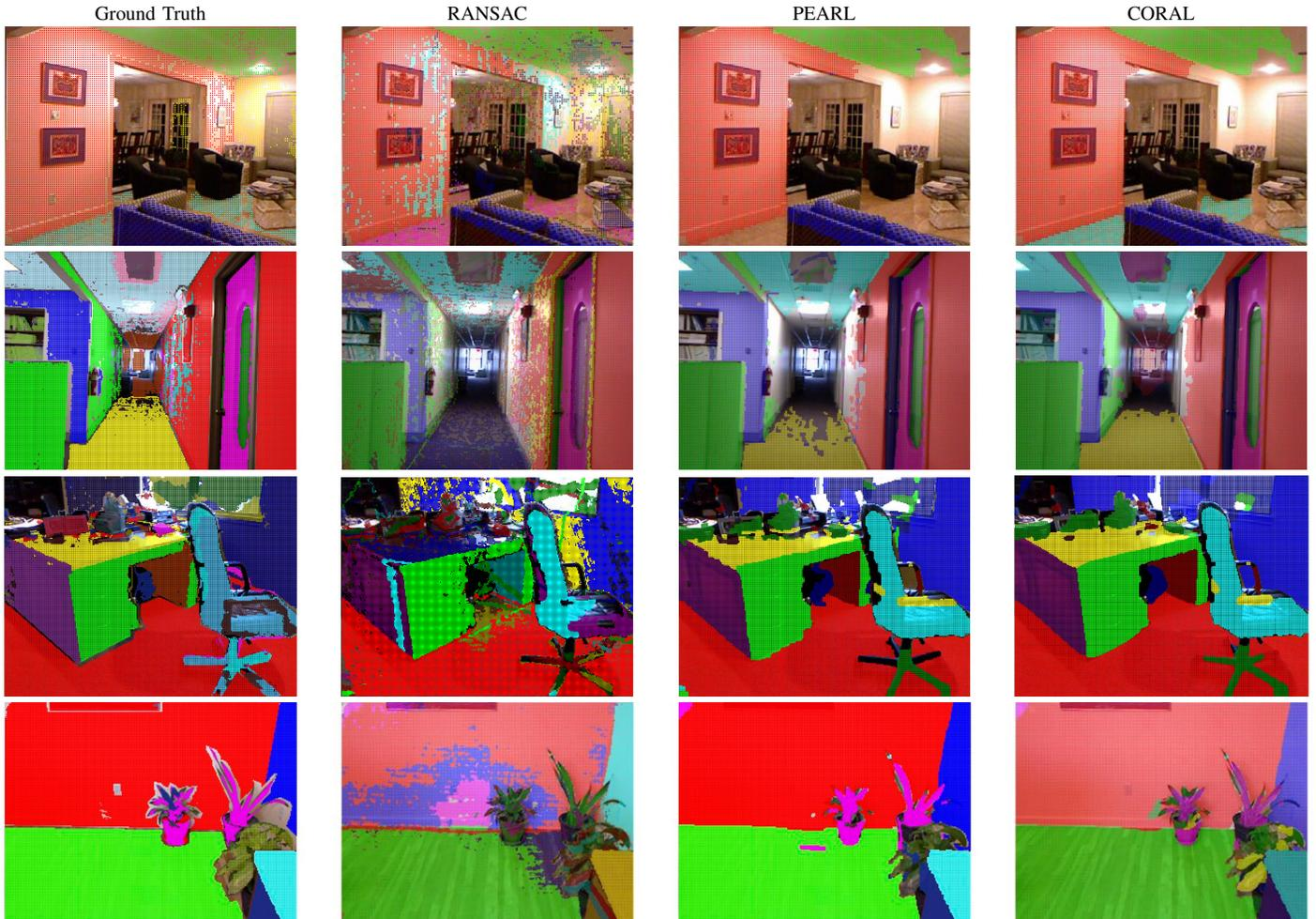
TABLE III: Plane segmentation on a sample of RGB-D images from the NYU-Depth dataset. with the Ground Truth, RANSAC, PEARL and CORAL results presented for each image. Pixel membership to a plane model is shown by superposing on a pixel a color-coded point that assigns it to a specific plane model.
