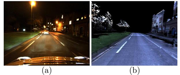
Figure 12. Failed localisation between a night-time dataset (a) and daytime prior (b). The localisation failed to converge for all images collected at night, due to the highly non-uniform illumination. A possible solution is a separate appearance prior collected at night, but this doubles storage requirements.
