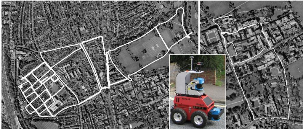
Fig. 2. Aerial map of the *Jericho* data set - 13.2 km, 16000 images (**Left**), and the *Oxford Science Park* data set - 3.3 km, 8536 images (**Right**). Vehicle trajectories are marked in white. **Middle**: *Marge* - our ATRV research platform
