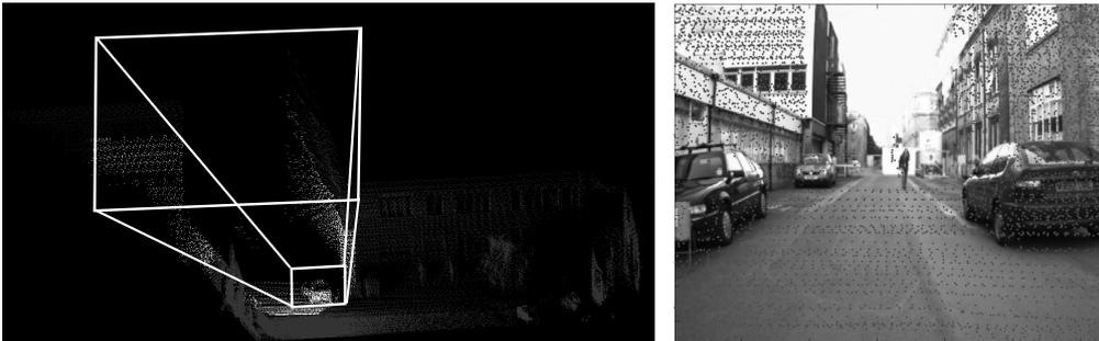
Fig. 4. Camera-laser cross-calibration. **Left:** A typical 3D laser point-cloud. Laser points within the camera frustum are highlighted (white). The frustum outlines have been added for clarity. **Right:** The respective 3D points (from within the frustum) as projected into the corresponding camera image.
