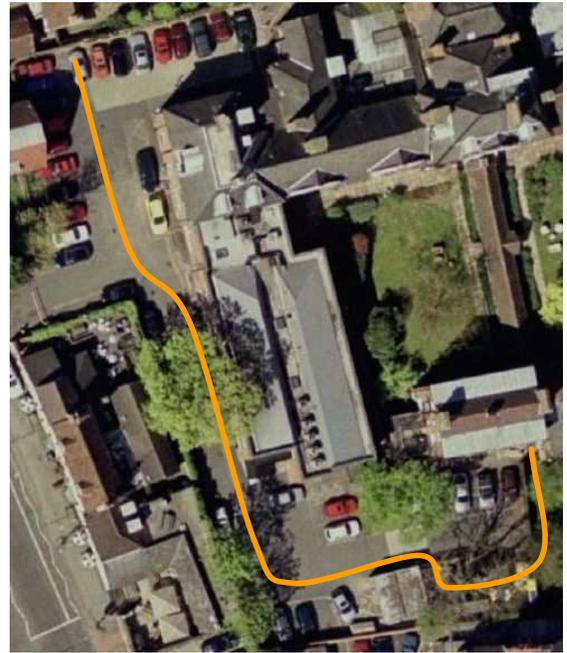
Fig. 4. Overhead of the teach trajectory (orange line). The urban environment offers a variety of features that affect the resulting localisation envelope, including wide open, narrow and asymmetric spaces.
