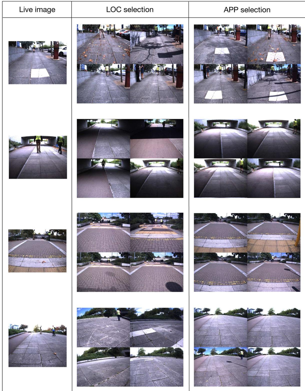
**Fig. 5.** Example images from a test route in Milton Keynes. The figure shows the live frame from a test traversal (left), a set of images that LOC selects for building the location-specific performance record (center) and a set of images that APP selects for the same purpose through experience-based navigation, the image-based localization system (right). Overall, the latter method results in a more accurate performance record.
