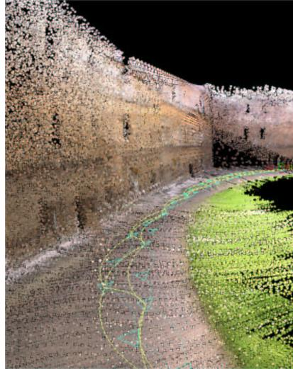
**Fig. 6.** Part of the 3D SLAM map shown in Figure 1 with the laser points painted with color extracted from the on-board camera. Black areas had no associated camera image.
