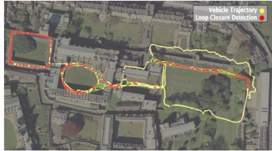
**Fig. 3.** Detected loop closures shown in red using the probabilistic loop closer (from [11]) described in Section 3. Loop Closures are plotted using low quality GPS data for ground truth.
