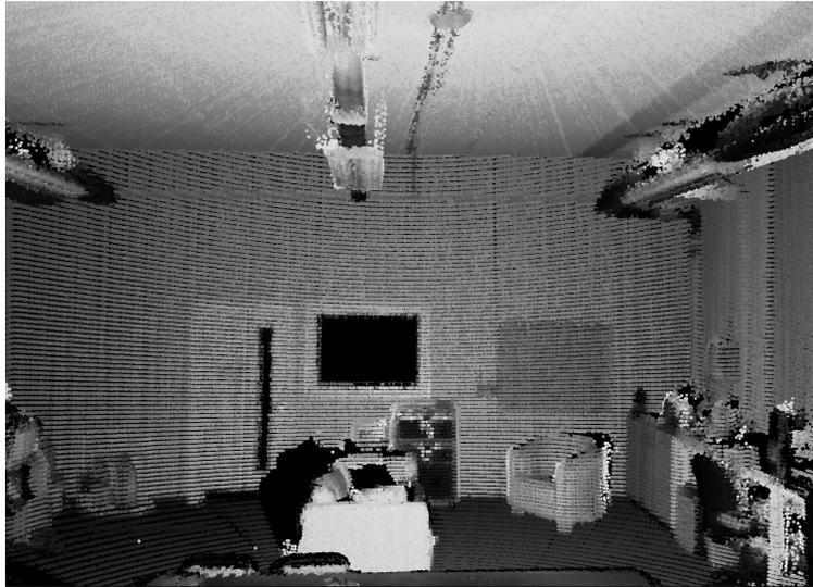
Fig. 8: A crisp point cloud of our lab generated using optimised values  $\hat{\Theta}$ ,  $\hat{\mathbf{H}}$ . Point colouring is based on laser reflectance values. This point cloud was achieved at a laser speed of 1HZ.
