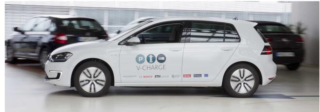
Fig. 1: The V-Charge VW e-Golf prototype performs fully automated navigation on parking lots using solely close-to-market sensors such as cameras and ultrasonic sensors.
