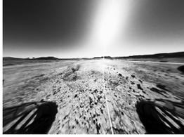
(c) Histogram equalisation can remove specularities caused by harsh glare.
