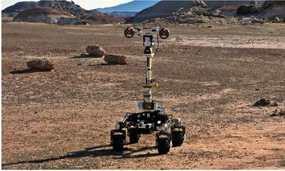
Figure 1. The Q14 Rover and PANCAM emulator. The PanCam is mounted at the top of the mast and can be rotated through 360 degrees and angled up/down using a mast mounted pan/tilt unit. The XB3 is the gold unit half way up the mast, the LIDAR is just below, and the Grasshopper is mounted on the front of the rover platform bed.
