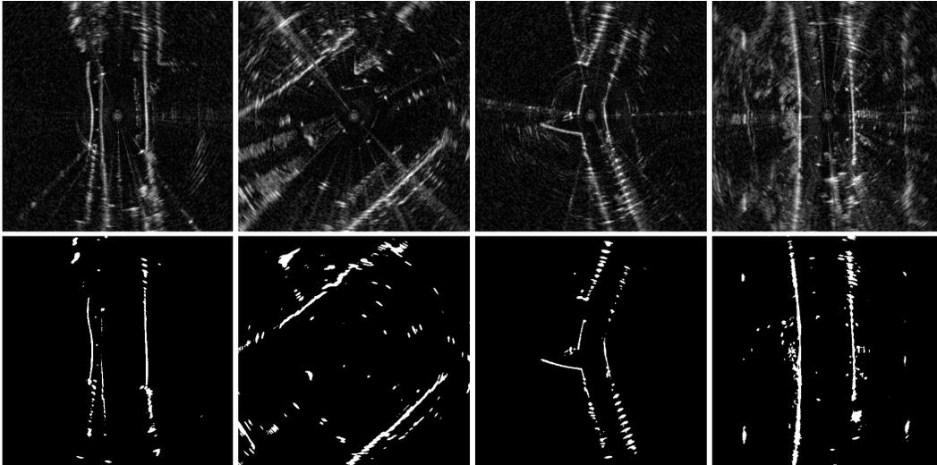
Figure 6: Example generated baseline masks used to supervise the radar masking network directly. For a given raw radar scan at time  $t$  (top) we can automatically generate high quality baseline masks identifying structure useful for pose estimation (bottom).
