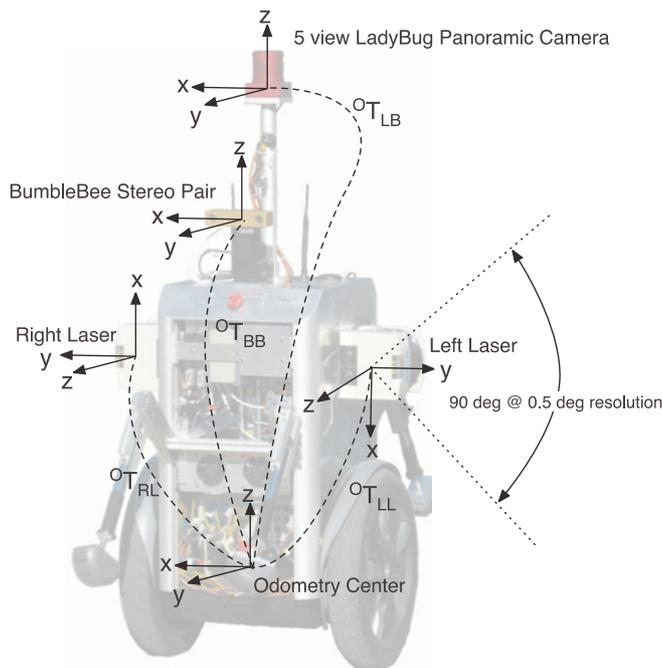
Fig. 2. Vehicle with sensor coordinate frame centres shown. Odometry data reports the robot centre position, taken to be  $y$ -forward and  $z$ -up frame anchored at the half-way point along the platform's wheel axle. The BumbleBee's coordinate centre is at the left camera's focal point and the LadyBug's centre is at the mean of the five radial camera centres. Laser scanner centres are at the point of intersection of the emitted beams.
